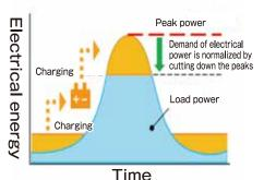
During the time period with small load such as holiday or night time, the battery energy storage systems is charged. During the time period when the load power concentrates, power is discharged, which cuts down the peaks of power.
