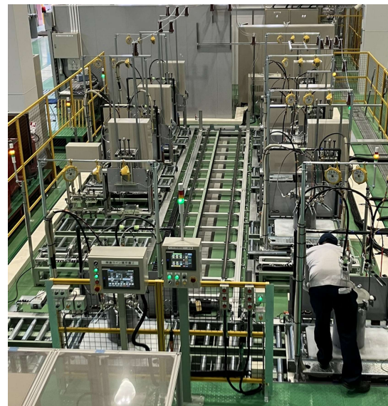
Consolidation of production functions and automation of core and inspection processes at the pole-mounted transformer factory => 22% improvement in productivity
