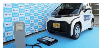
Wireless charging system for ultra-compact electric mobility vehicles
