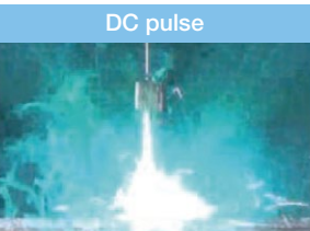
DC pulse Welding current: 80 A Wire feed rate: 5.2 m/min Welding voltage: 17.8 V
