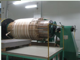
Transformer coil in front of an insulated wall
