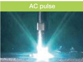
AC pulse Welding current: 80 A Wire feed rate: 5.9 m/min Welding voltage: 17.8 V EN ratio: 20%
