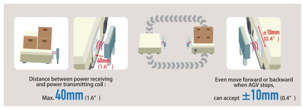
AGV alignment mechanisms or guide rails are unnecessary.
