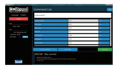
When changing line layout, AGV operation method, or battery, it is possible for customers to change charging parameters such as charging current and full-charge voltage by themselves.
