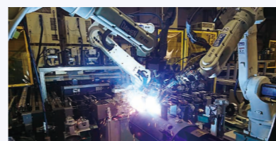
Automated welding of pole-mounted transformer cases
