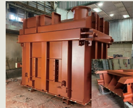
Transformer casing during paint drying process
