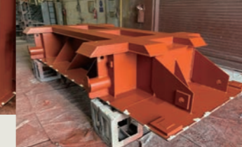
Transformer base during paint drying process
