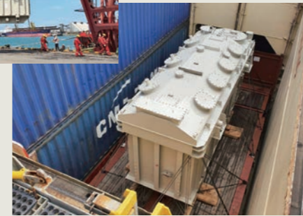
Transformer stowed onboard a container ship
