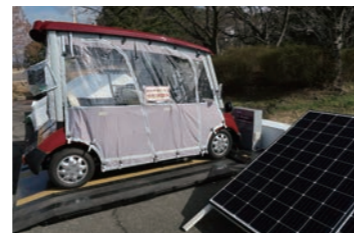
EV being charged on the “D-Broad EV® Charging Dock”
