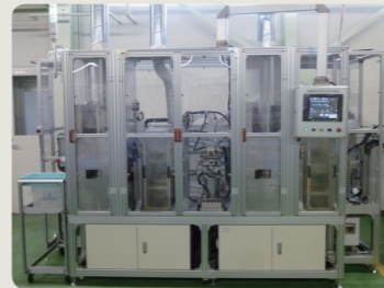
Efficiency enhancement by automating soldering process of heat storage fuse elements
