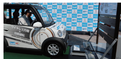
Charging using the “D-Broad EV Charging Dock”
